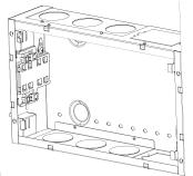
**Note:** You cannot mount vertically in new installs. To mount vertically, the dog ears must clasp the drywall.
